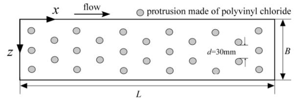
Figure 2. An arrangement of protrusions
